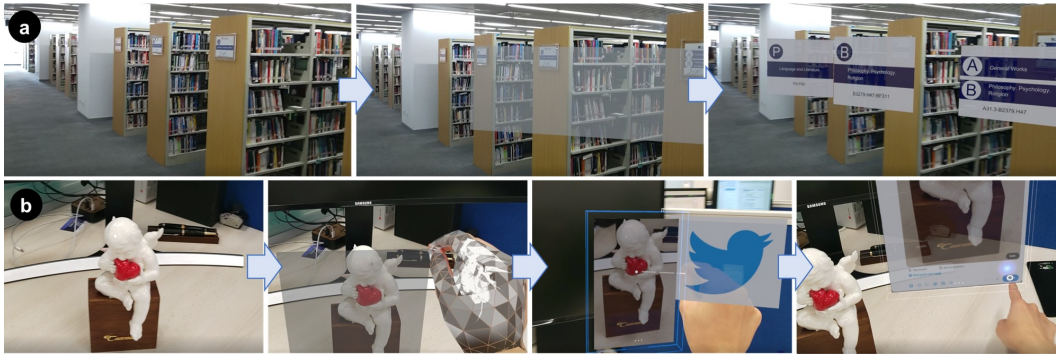
Fig. 5. Two example application scenarios with region selection via an AR HMD. (a) Information retrieval for the book categories in a library. (b) Capturing an interesting part of a user's view and sending the captured part to another application.
